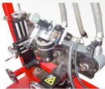
Ergonomically arranged flux recovery belt assembly with Lincoln NA3S weld head
